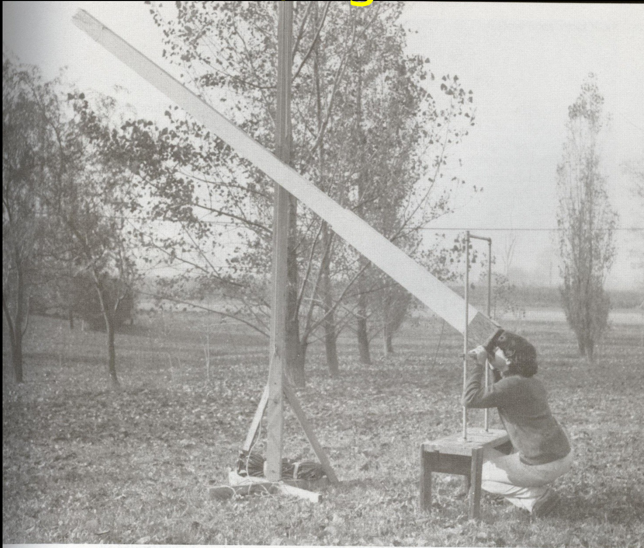
Modern version of a seventeenth-century long-focus refractor in use. The aperture of the lens is 2.2"; its focal length is 168'.
