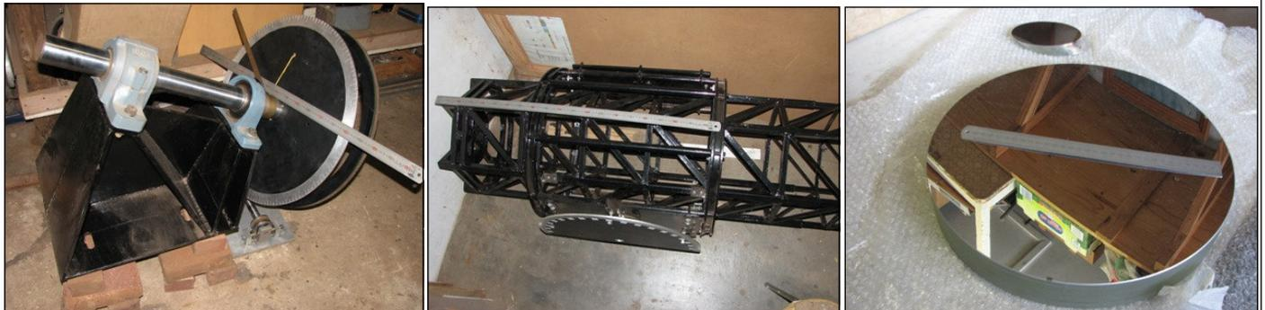
Photographs of parts of the telescope-to-be, left to right: **1.** The RA shaft with setting circle and 600mm diameter worm gear. **2.** The tube with the declination cage allowing the tube to be rotated. **3.** The precious optics, with the metal ruler on the surface, which nearly induced a heart attack in some members of the audience. I trust that Pierre will be more careful about what he places on top of the mirror in future.
