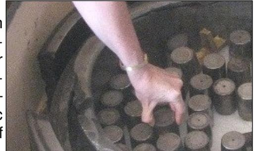
The photograph on the left shows the damaged main bearing after removal from the telescope. The cylindrical rollers were originally positioned between the two big concentric cylindrical rings. The photograph on the right gives an idea of the size of the bearing.
