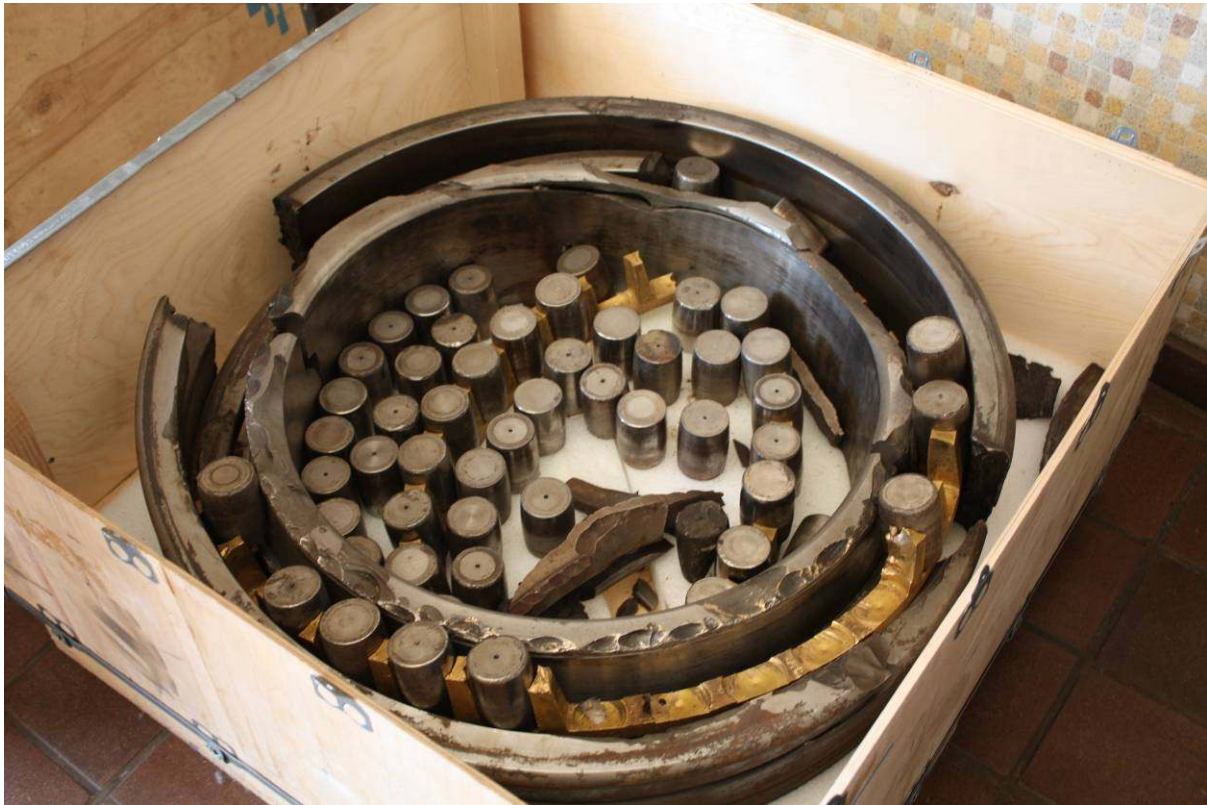
The broken bearing from the 26 meter radio telescope.
